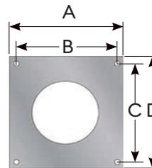
A support must always be used above an Adjustable Length where applied in a vertical application, or where the Adjustable Length would be otherwise liable to load. The maximum length which can be supported by this component is 30 metres.
